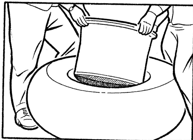
Figure 2-17 Lifting Wheel out of Tire
