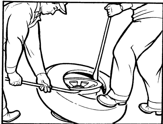
Figure 2-26 Prying Bead over Wheel Flange
