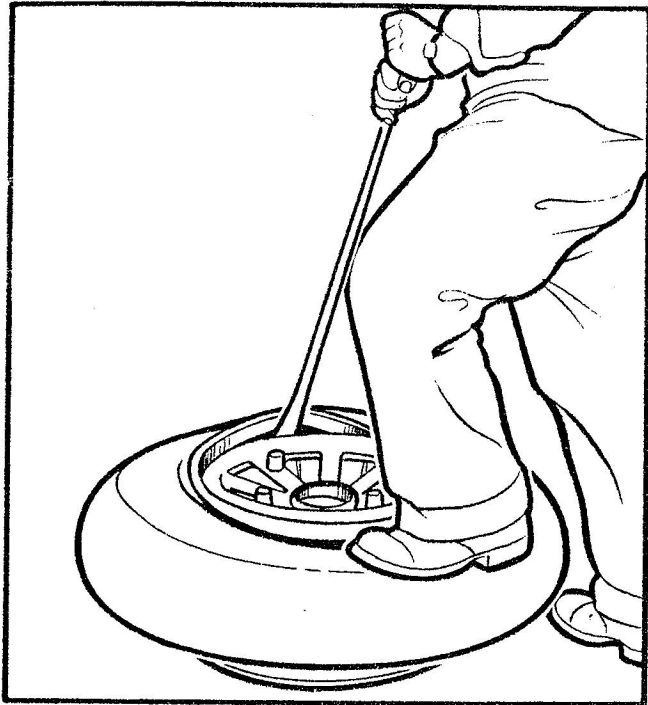
Figure 2-27 Prying Bead into Wheel Well
