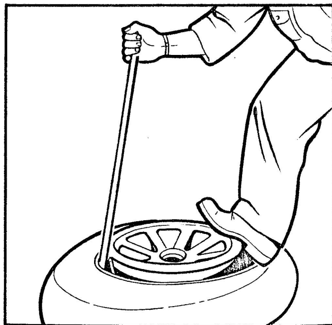
Figure 2-6 Prying Bead up at Valve
